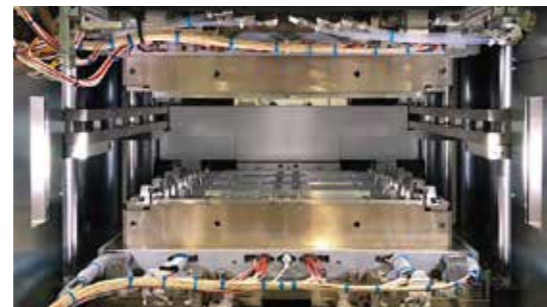
Molding press and molds for next-generation semiconductor package
