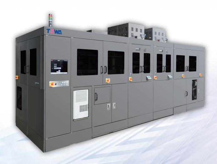
Transfer molding system for 2.5D/3DIC/Chiplet products
