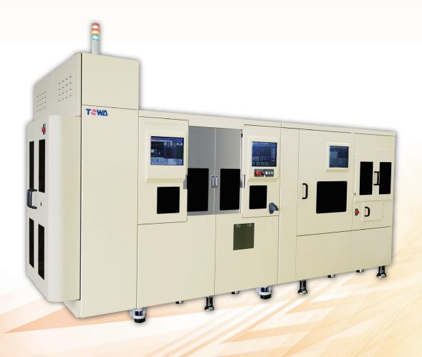
Singulation system for cutting substrates
