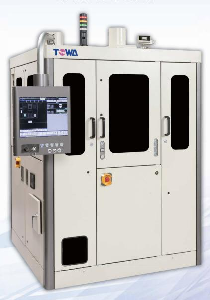
Transfer molding system suitable for small volume production of multiple products
