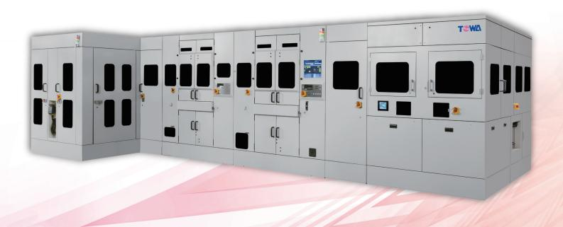
Compression molding system for large size PLP molding to meet industry needs
