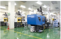
Fine plastic products are all manufactured in cleanrooms, with more than 40 electric injection molding machines in place.
