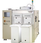
Wafer marker for laser marking on wafers with product names, lot numbers, and other control numbers
