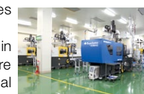
Fine plastic products are all manufactured in cleanrooms, with more than 40 electric injection molding machines in place.
